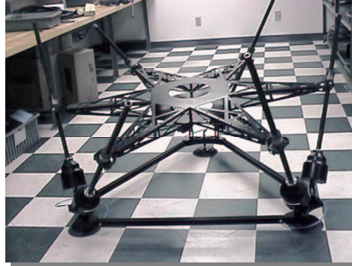
Figure 1. First Generation STARC Stewart Platform Manipulator
